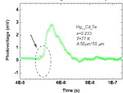
Fig 3 Photoresponse profiles from MCT photodiode with the Cd composition is 0.233.
