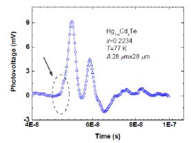
Fig 4 Photoresponse profiles from MCT photodiode with the Cd composition is 0.2234.
