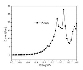
Fig. 3. The I-V characteristics for reverse bias under dark.
