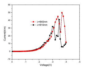
Fig. 4. The I-V characteristics for two wavelengths of 810 and 840 nm.
