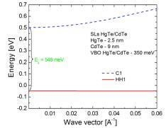
Fig. 2. Typical dispersion relation for C1 and HH1 in growth direction for HgTe/CdTe SLs at T = 155 K, VBO = 350 meV.
