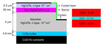
Fig. 1. Simulated nBn HgCdTe structure with HgTe/CdTe SLs barrier.
